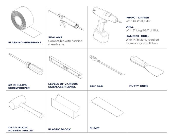
\*Except in circumstances where a particular shim type is specified by applicable building codes – either wedge shims or horseshoe shims may be used. Shimming must be even across the door unit. Each shim must be long enough to cover the full width of the door frame from front to back.
