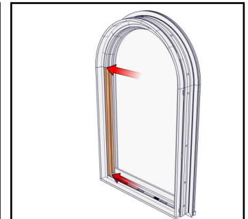
RT Jamb Cover Install
