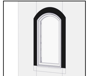
Flashing Over Flange
