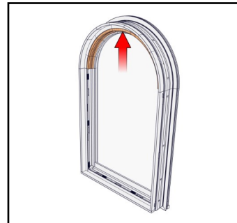
RT Head Cover Install
